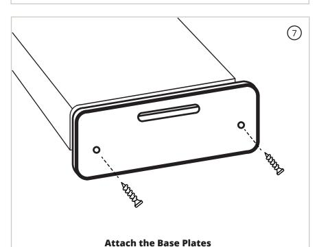
Align each base plate with the holes in the feet and securely fasten.
